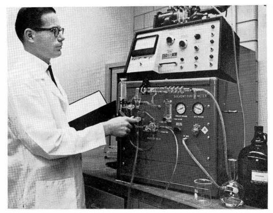
R. C. MARSH of Manufacturing Research Division 2564 demonstrates a new cleanliness test meter which rapidly detects and continuously measures contamination levels in volatile cleaning solvents. Levels as low as one part per million can be easily measured.
